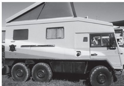
From top. 1: Swiss Bucher Duro with a 4-tonne payload and a six-litre, 250-hp Cummins. 2: From Italy, an older Bremach Xtreme with an Iveco engine. 3: Their newer T-Text model running various 3-litre CRD Fiat engines. 4: An old 6WD Pinzgauer, probably with a 2.4 VW engine. All a bit narrow inside but this Pinz has an elevating roof.
