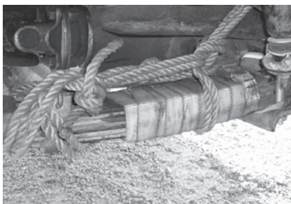
Binding broken leaves together can limit stresses spreading to other leaves and can even work if the main leaf is broken.
