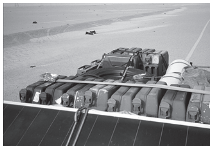
An 80-watt panel makes a handy spoiler for a rack of jerries.
