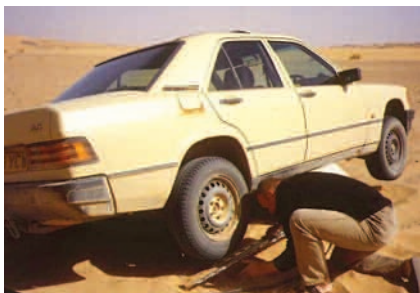
Airbag jack easily lifts car without damage.
