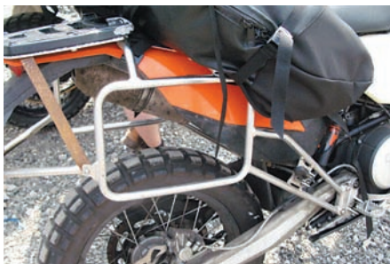
Left: Footrest-mounted KTM rackangle. Note rusting brace added from the tail rack.
