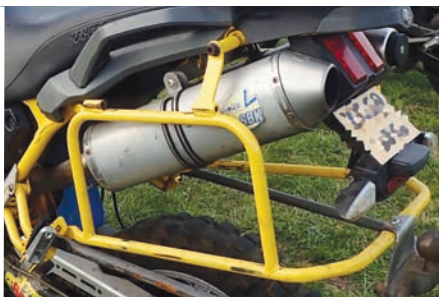
Left: Footrest-mounted KTM rackangle. Note rusting brace added from the tail rack.
